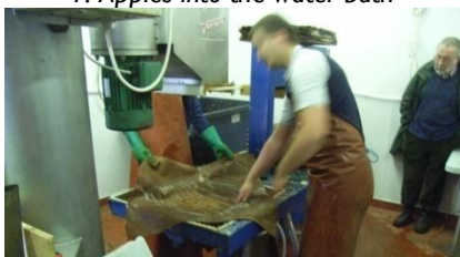
2. Cloth laid out between boards
